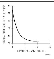
FIGURE 7.  $\theta_{(J-A)}$  vs Copper (1 ounce) Area for the TO-263 Package
