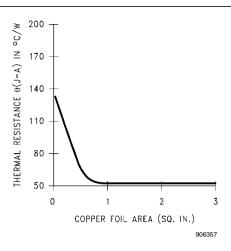
FIGURE 5.  $\theta_{(J-A)}$  vs Copper (2 ounce) Area for the SOT-223 Package
