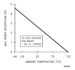
FIGURE 8. Maximum Power Dissipation vs T<sub>AMB</sub> for the TO-263 Package
