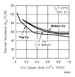
FIGURE 9.  $\theta_{\text{JA}}$  vs 2oz Copper Area for TO-252
